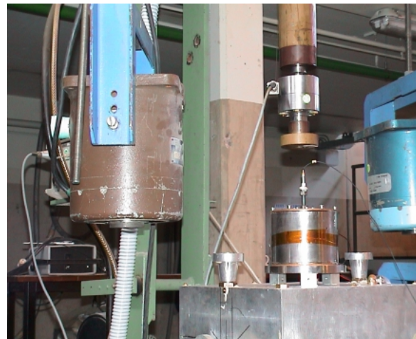
Fig. 5b. 400N TNO actuator in comparison with 200 N Derritron shakers.
