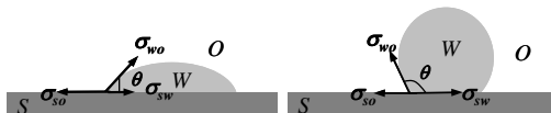
Figure 1. Contact angles set up on solid substrates. Water and oil on a hydrophilic surface (left) and a hydrophobic surface (right). W, O and S indicate water, oil and solid, respectively.
