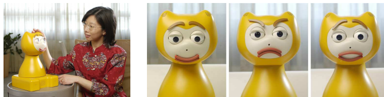
Figure 1: Left: The iCat has various sensors including touch, vision and sound sensors to perceive our physical world with. Right: The iCat is able to show various facial expressions. From left to right: happy, angry and surprise.
