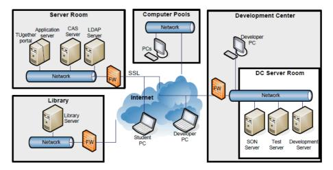
Figure 2: TUgether portals IT architecture. (FW: Firewall, DC: Data Center, CAS: Central Authentication Service, SON: Personal Development Server.)
