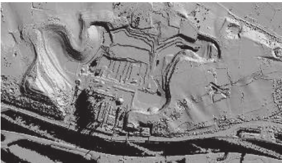
Figure 2.24 Pictorial representation of a digital surface model of the Sint Pietersberg open-pit mine in the Netherlands. The size of the pit is roughly 2 km × 1 km. The terraced rim of the pit is clearly visible. The black strip near the bottom of the image is the River Meuse. Courtesy Survey Department, Rijkswaterstaat.
