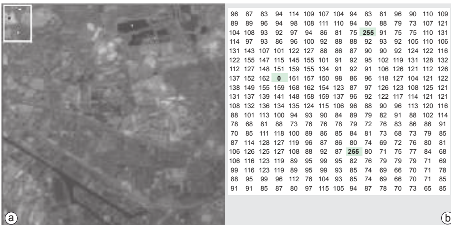
Figure 5.21 Image with spike errors (a) and the DNs (b).
