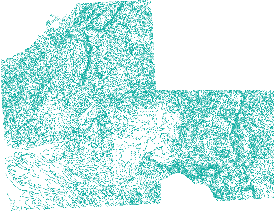
Figure 8.16 A vector-based elevation field representation for the Falset study area; see Figure 8.1. Elevation isolines are indicated at a resolution of 25 m.
