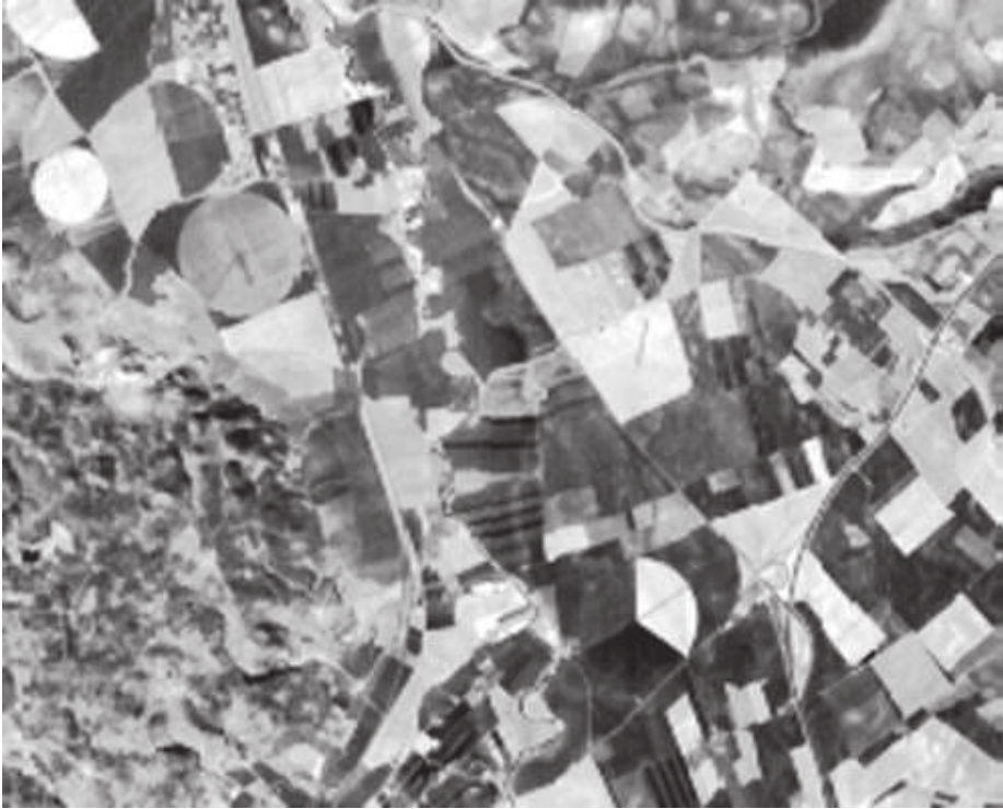
Figure 6.1 RS image of the Antequera area in Spain; the circular features are pivot irrigation systems. The area imaged is 5 km wide.
