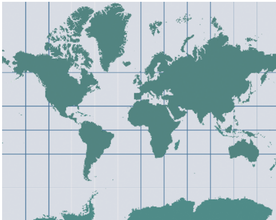
Figure 3.19 The Mercator projection, a cylindrical map projection with conformal properties. The area distortions are significant towards the polar regions.
