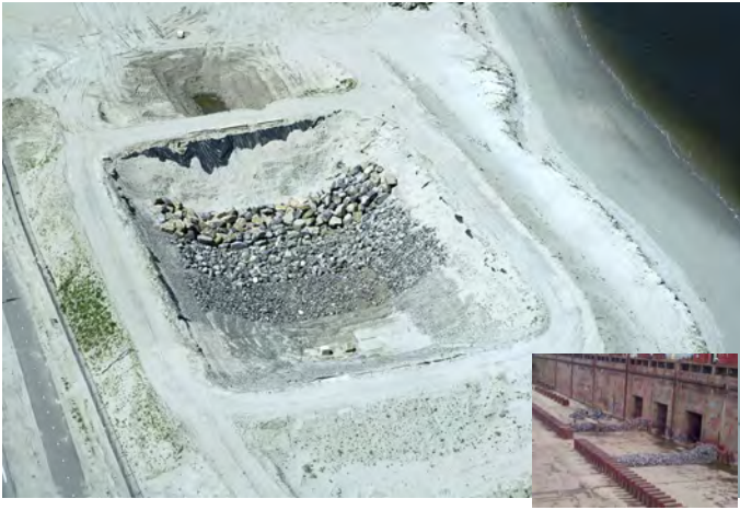
Figure 1: Trial set-up in the test-pit at the Maasvlakte port extension with 20-135 mm (including 4 objects), 5-70kg, 150-800 kg and 1-10t gradations. Inset: Trial set-up in the Verolme dock (1999).
