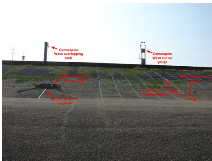
Figure 2: Measurement configuration in the Petten transect (left, a) and on the dike (right, b).
