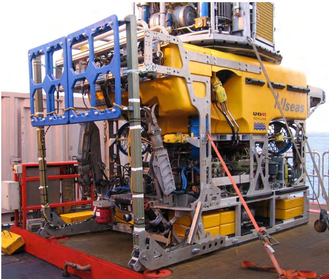
Figure 1: April 2012 - ROV with INS mounted on survey skid
