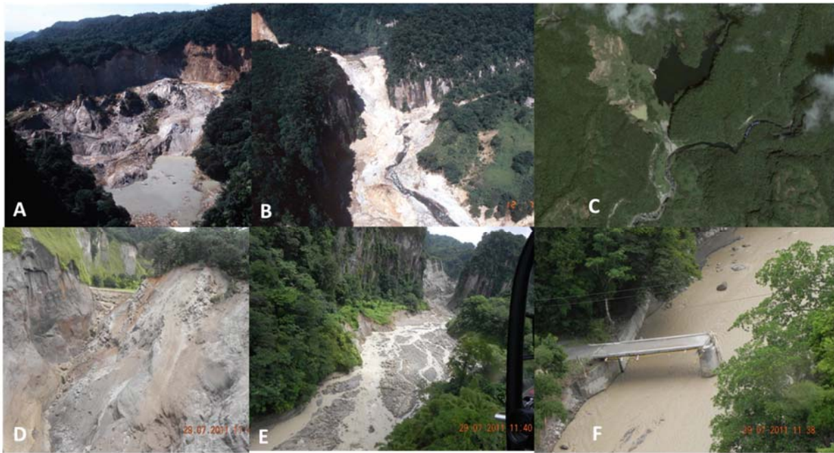
Figure 4-11: Mathieu landslide dam development. A: Carholm landslide blocking the Mathieu River and forming a lake in 1997 (Photo: J. DeGraff), B: View from downstream along the Layou valley towards the confluence of Layou and Mathieu river, with landslide dam location in 1997 (Photo: DeGraff, 1997); C: Google Earth image 3/8/2005 showing dammed lake. D: landslide dam washed out after dam break in May 2010; E: View from downstream towards former landslide dam, note the large area affected by dam break flooding; F: Bridge destroyed by dam break flood.
