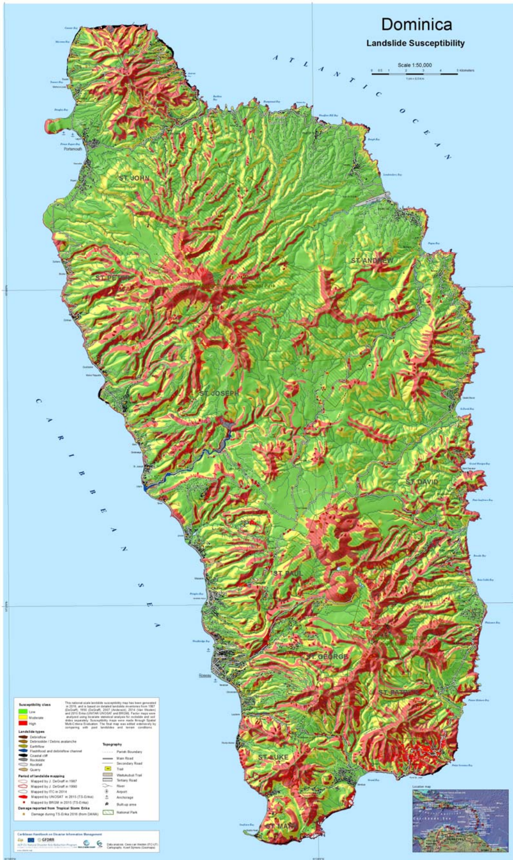
Figure 6-25: Final landslide susceptibility map for Dominica. The full map can be downloaded as pdf from the following website: http://www.charim.net/dominica/maps
