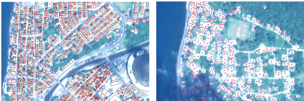
Figure 8-1. Example of the building extraction as points for the whole island of Dominica. Left: example for the centre of Roseau for which also building footprints were available show a good correlation. Right: example from Pointe Michel.
