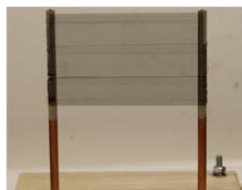
Figure 1: A super-aligned CNT film placed across two copper electrodes
