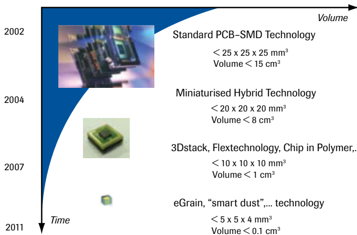
Figure 12 System integration roadmap for the coming decade: the development of 3D stacking technology, flex technology, and full wafer-scale 3D integration will lead to two orders of magnitude reduction in volume and enable smart unobtrusive autonomous sensor systems
