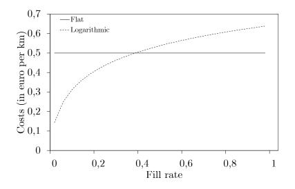
Figure 10: Flat and logarithmic cost functions, providing a transportation cost per km based on the container fill rate.
