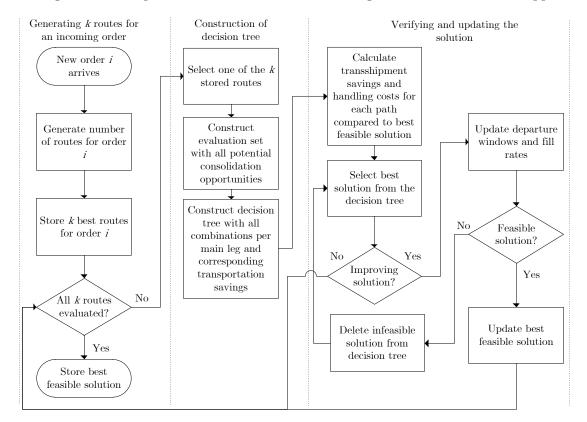
Figure 2: Flowchart with the main steps of the consolidation algorithm. The algorithmic procedure for each column is outlined in the subsequent sections.
