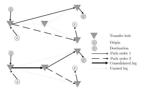
Figure 1: Example of the consolidation of two orders. The top panel illustrates the individually least expensive routes for both orders. The bottom panel shows how consolidation reduces the total travel distance, but introduces additional handling operations as well.
