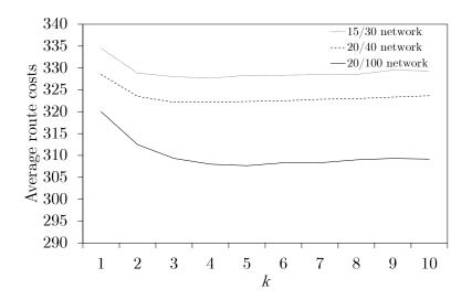
Figure 13: Average route costs for three semi-random networks, measured for  $k = \{1, 2, ..., 10\}$ . It can be seen that the network containing 20 hubs and 100 main legs benefits most from the algorithm, due to the higher variety in good routes.
