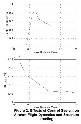
As a further step a number of load cases were investigated by the aircraft loads specialist to analyse the effect of the yaw damper on the fin structure loads. The influence of the yaw damper on the fin loads strongly depends on the yaw damper gain (figure 2).
