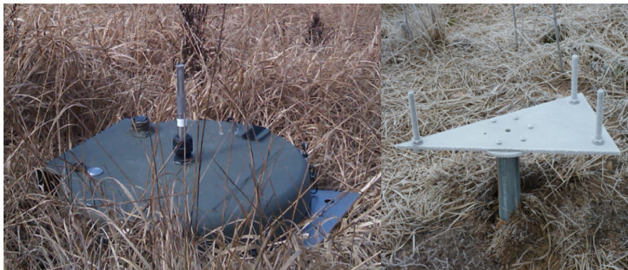
Fig. 4. Left: Unattended Ground Sensor without its windshield. Right: Sensor post.
