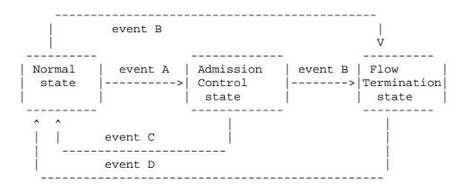
Figure 4: States of operation, flow termination with congestion notification based on probing
