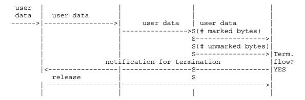
Figure: 3 LC-PCN Flow Termination handling
