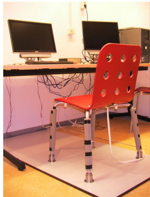
Figure 1: Pressure sensitive chair used for the measurement of people's changes in sitting position.
