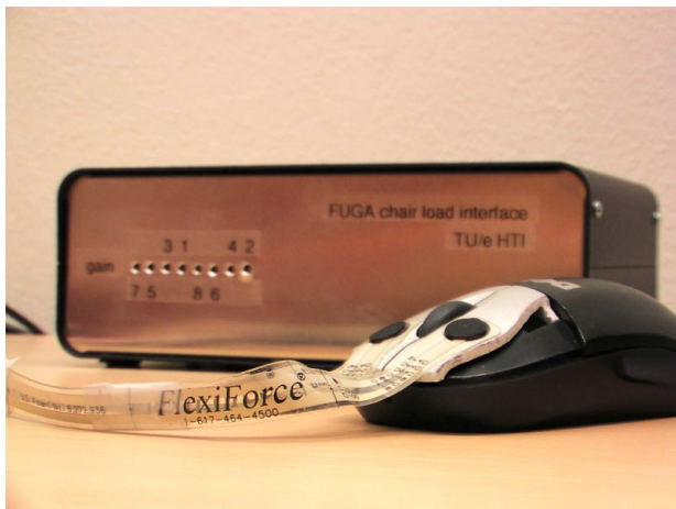
Figure 2: Pressure sensitive mouse measuring force applied to the mouse during game-play.
