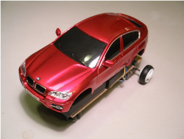
FIGURE 1. 1:24 SCALE VEHICLE USED IN TEST BED
