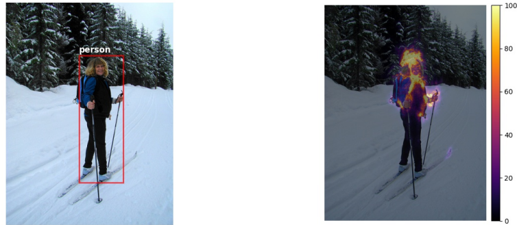
Fig. 36. A person detection made by the detector (left). An explanation for the person y_left_top coordinate prediction (right). The most of the important pixels highlight the object detected. In addition, the explanation is coherent with the bounding box coordinate as the explanation highlights region near the y_left_top .
