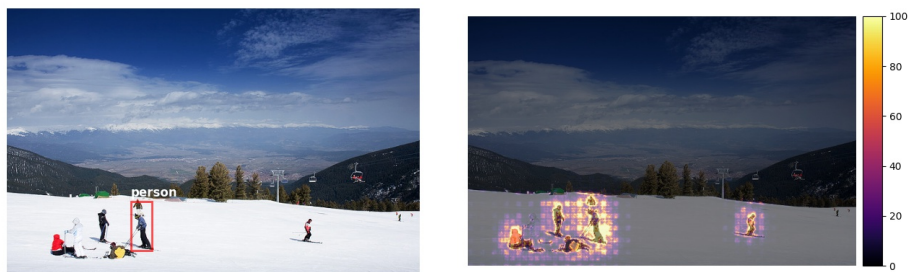
Fig. 37. A person detection made by the detector (left). An explanation for the person x_right_bottom coordinate prediction (right). The important pixels highlight the object detected. However, the explanation highlights numerous pixels outside the the detected object and is highly noisy.
