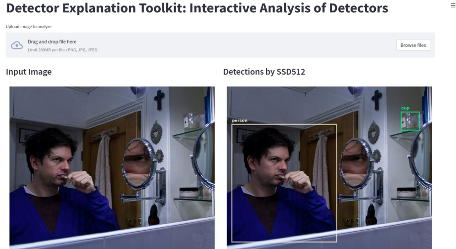
Fig. 41. Illustration of the input image user uploaded by the user (left) and detections (right) made by the SSD512, the detector selected by the user, in the input image. The detectors available for off the shelf analysis are EfficientDet-D[0-7, 7x], SSD512, and Faster R-CNN.
