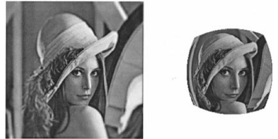
Fig. 4. Foveated image in Cartesian coordinates (left) and curvilinear coordinates (right) [14]
