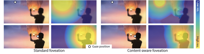
Fig. 5. Ordinary foveated rendering techniques (left) using a fixed quality decay for peripheral vision. While this can be a conservative solution, it does not provide a full computational benefit. [17] performs content-adaptive foveation (right) and relaxes the quality requirements for content for which the sensitivity of the human visual system at large eccentricities degrades faster [17]
