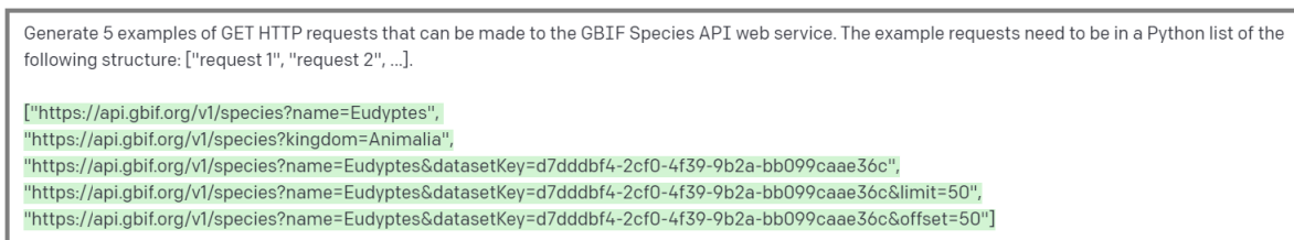
Figure 18: Example of the text-davinci-003 model returning a response in a Python list, as specified in the prompt.
