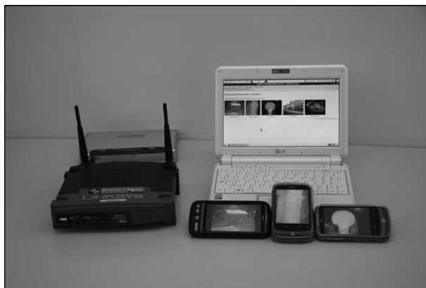
Figure 6. An example photomathon toolset for collecting photos from a set of Android mobile phones, comprising of a wireless router, a netbook computer and some phones.
