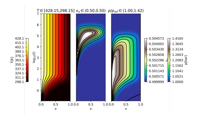
Figure 2: Relaxation of system (B.1) after temperature step of the boundary condition ( $\Delta T = 130$ K). The Dirichlet boundary conditions for the pressure p and the molar fraction  $x_a$  are constant and equal for the both boundaries.
