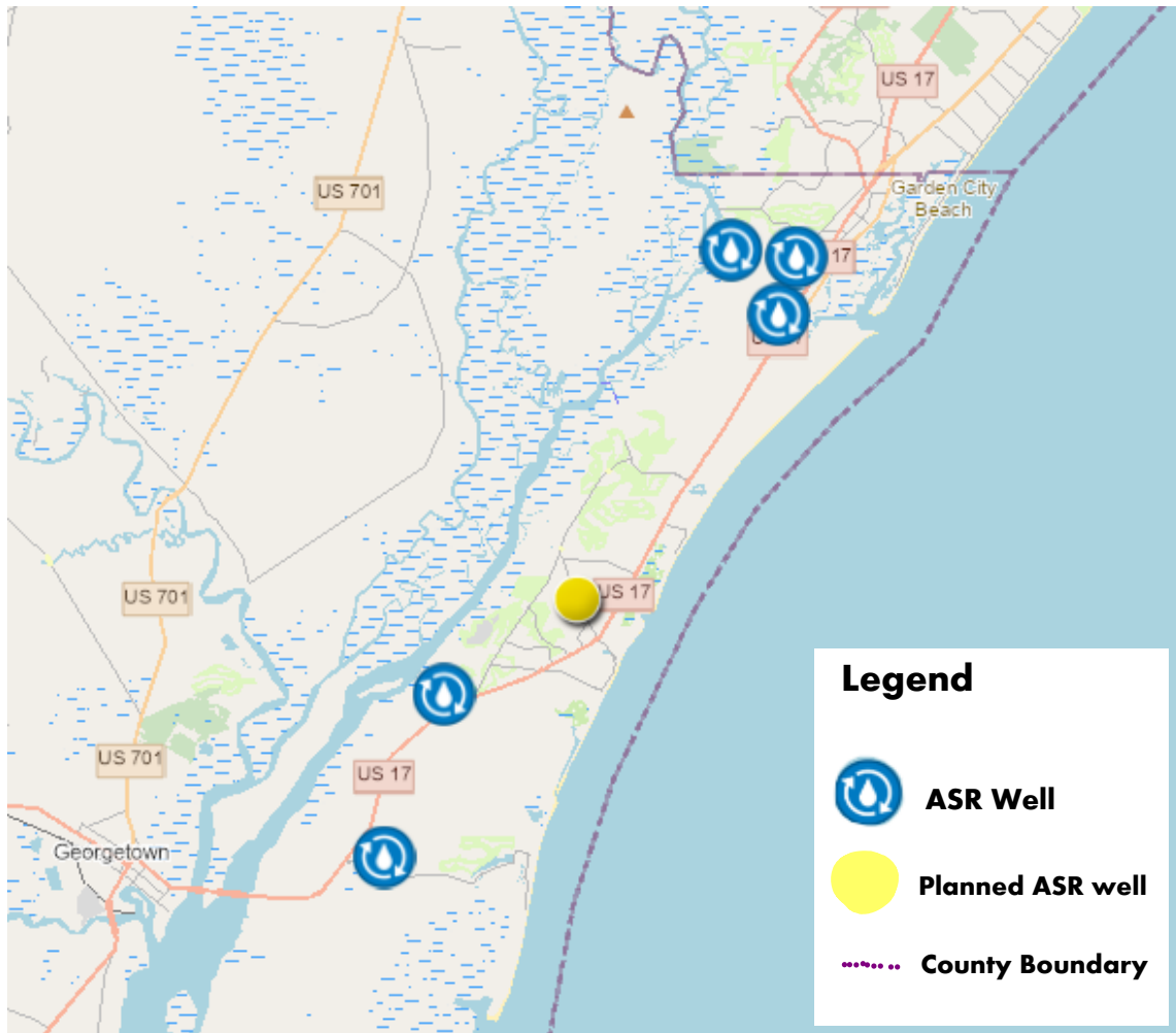
Figure 2: GIS map showing the extent of the Waccamaw Neck region in Georgetown County. Within this region there are five ASR wells (shown in blue) and one planned ASR well (shown in yellow).
