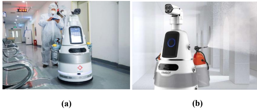
Figure 1-4 A spray liquid disinfection robot [17] (a) Robot moving in hospital.(b) Robot spraying liquid agent.
