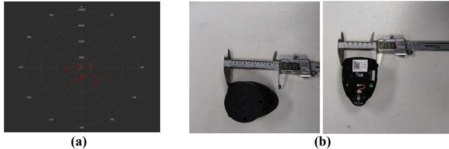
Figure 3-12 (a) 2D lidar point cloud (b) A1M8-R5 single-line lidar
