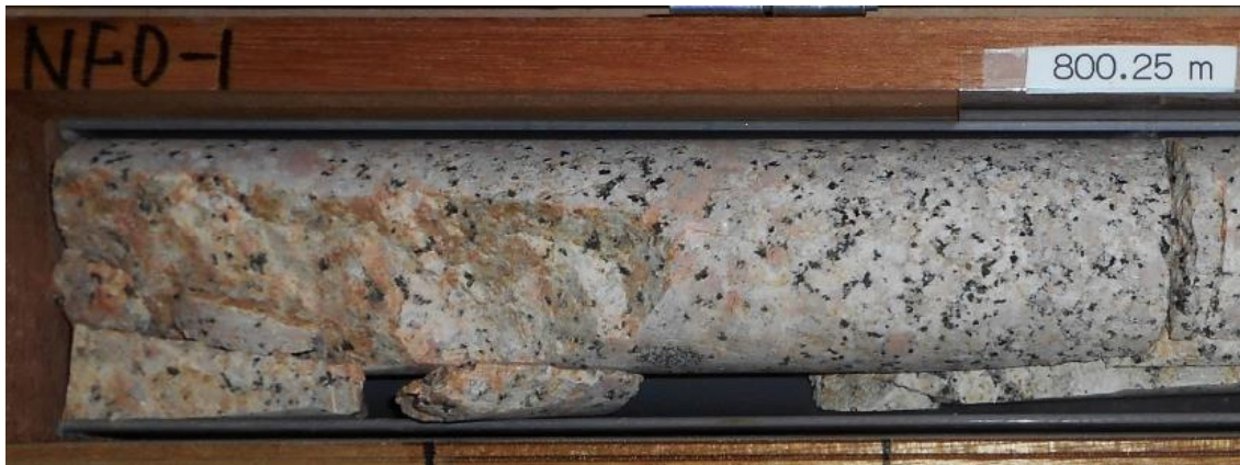
Figure 4-8. NFD1 800 core. The outer periphery was removed and only the centre was used for luminescence measurements.
