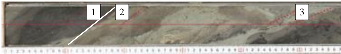
Figure 4-5. NFD1 S2 core. The line between 1 and 2 is considered to be the gouge.
