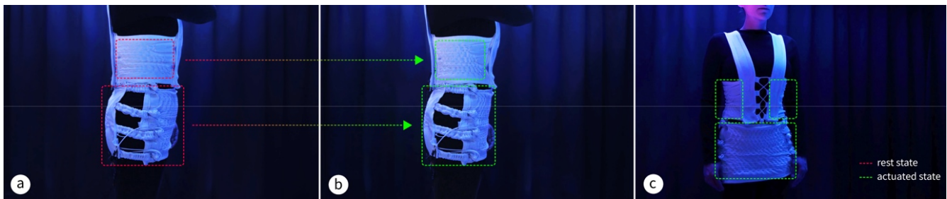
Figure 12: One of the audience members wearing the Corsetto after the first performance took place; (a) side view at rest state; (b) side view of actuated ribs and abdominal modules; and (c) front view of actuated ribs and abdominal modules compressing onto the torso of the listener by ~18 %.
