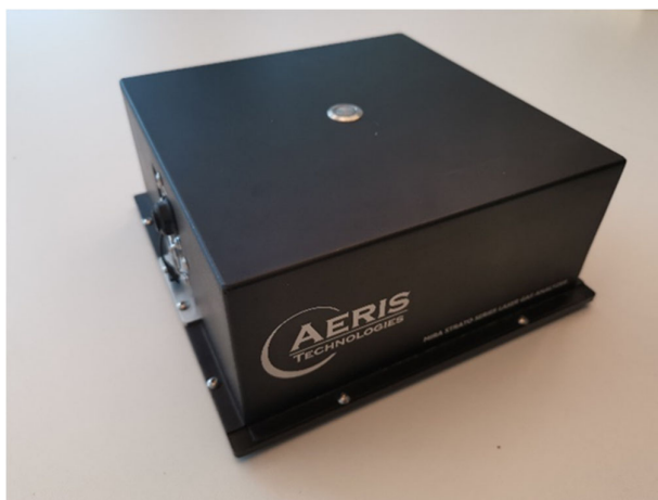
Figure 1. The laser spectrometer used measures methane and ethane with 1 ppb sensitivity at 1 s time resolution. The data are transmitted to the ground via radio modem and shown in real-time on a computer.
