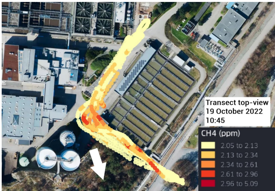
Figure 17. Example of a drone-based methane measurement at the primary clarifiers of the WWT plant on October 19, 2022, carried out at 14:31. In the upper graph The height of the curves corresponds to the concentration of the measured gas at ground level (above background concentration). The highest measured methane concentration at this measurement was 301 \mu\text{g}/\text{m}^3 . See Figure 3 for a general description of the graph structure. Map: Google Earth™ © 2022. The lower graph visualizes the flight path of the drone as seen from above. Graphic from: www.kepler.gl © with underlying Map from Mapbox©.
