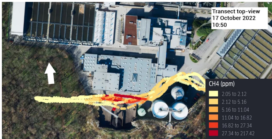
Figure 20. A typical example of a "wall transect" downwind of the sludge piles at the WWT plant on October 17, 2022. These transects were carried out at various heights, from 0m to 50m. The spheres indicate methane measurement points, and each colour indicates absolute concentration in ppm above background level. White arrow indicates wind direction. Map: Google Earth™ © 2022.. The lower graph visualizes the flight path of the drone as seen from above. Graphic from: www.kepler.gl© with underlying Map from Mapbox©.
