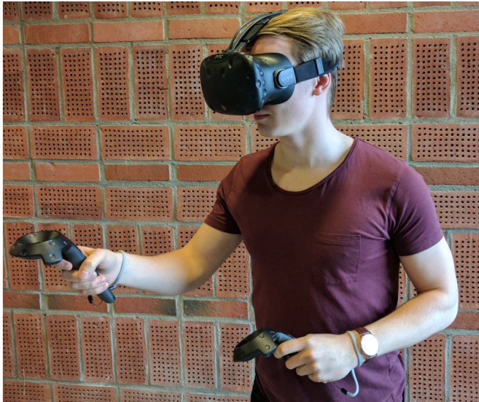
(a) A figure showing a person wearing a VR-headset consisting of an HMD and two hand-held controllers.
