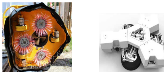
Figure 22. Example of commercial cleaning device with capture. To the left brush with suction propeller and sealing (rubber edging) . To the right high pressure waterjet with magnetic attachment (Fleetcleaner)
