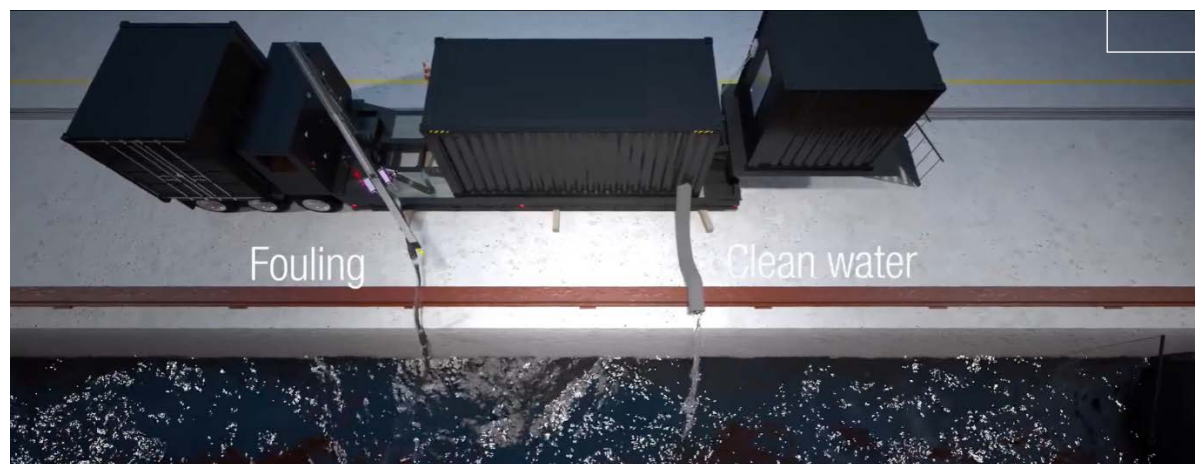
Figure 24. Filtering setup on shore with discharge of filtered water back to sea (ECOsubsea)
