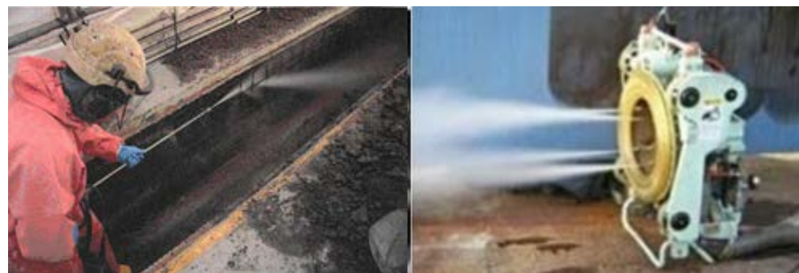
Figure 15. Non cavitation water jet system (left)[2], High-pressure water cleaning jet technology (right) (HullWiper)
