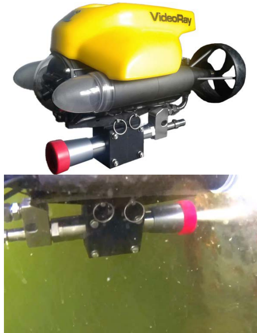
Figure 14. Waterjet cavitation cleaning with ROV ( DiveWise )
