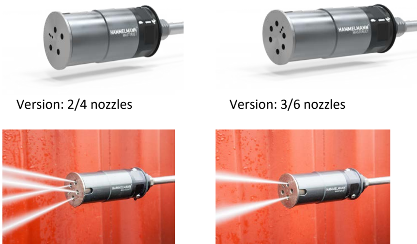
Figure 13. Example of water jet tips for underwater hull cleaning. Different nozzle configurations operate under pressure 1800-3200 bar and flowrate up to 60 LPM (Hammelmann)
