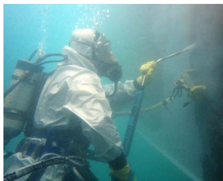
b) Niche area cleaning using waterjet
