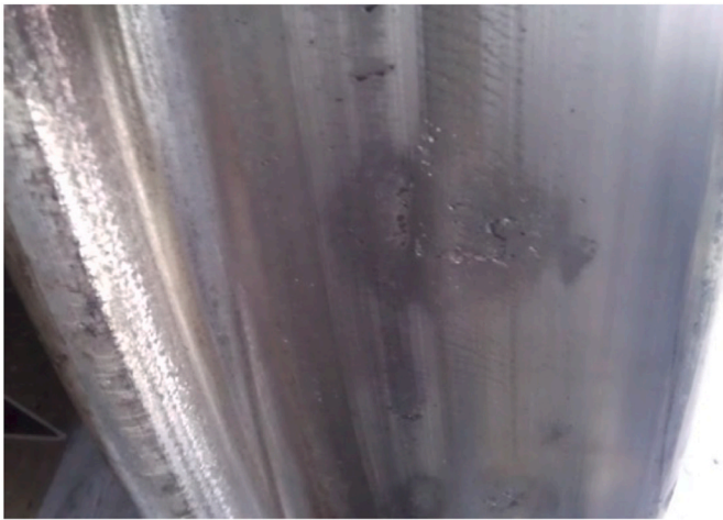
Fig. 5. Thermal facets (dark regions) on top of bands of surface initiated RCF.
