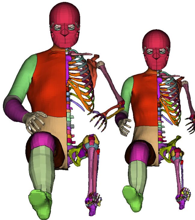
Figure 8. SHBM as parametrically morphed to (left) male, 189 cm, 127 kg, 35 years, (right) female 151 cm, 52 kg, 35 years. Skin parts hidden to show skeleton.
