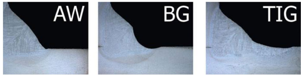
Fig. 1 Weld profile in as-welded, burr ground, and TIG-dressed states [4]
