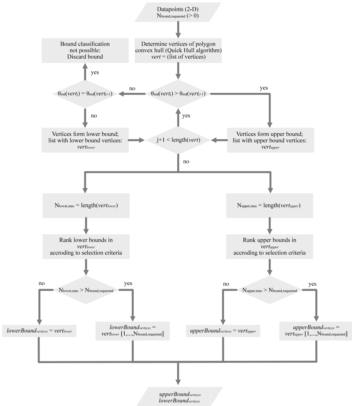
Fig. 5. Algorithm to identify a predefined number of upper and lower boundary functions for 2-dimensional data. Note that counter-clockwise order of the vertices of the polygon convex hull was assumed.
