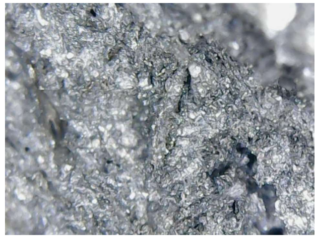
Figure K1: a) magnified image of 100-0 clay-sawdust ratio surface b) magnified image of 55-45 clay-sawdust ratio surface.
