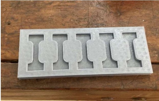
F1: Dogbone mould for the tensile strength testing of PDMS samples.
