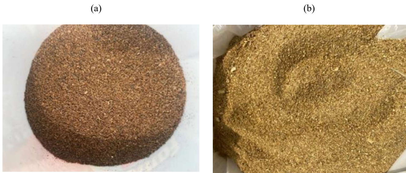
Figure 3.8: Sample Preparation: (a) Sieved Banana Peels and (b) Sieved Orange Peels.
