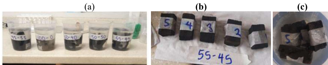
Figure 3.17: Determination of Porosity and Density: a) set-up of samples in water, b) saturated samples, and c) saturated samples left on paper towel for droplets of water to dry before measurements.
