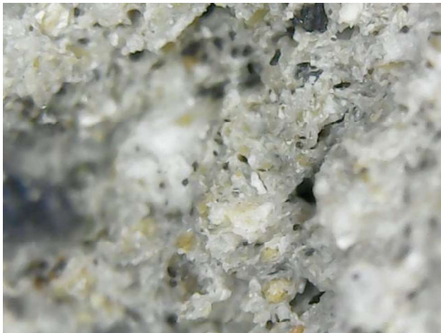
Figure K1: a) magnified image of 100-0 clay-sawdust ratio surface b) magnified image of 55-45 clay-sawdust ratio surface.
