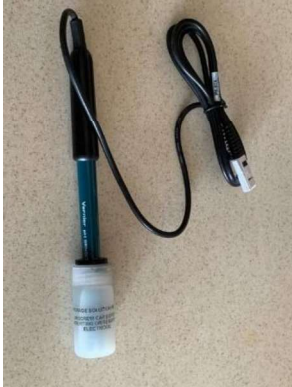
H1: (a) pH sensor (b) turbidity sensor (c) Conductivity sensor (d) temperature probe
