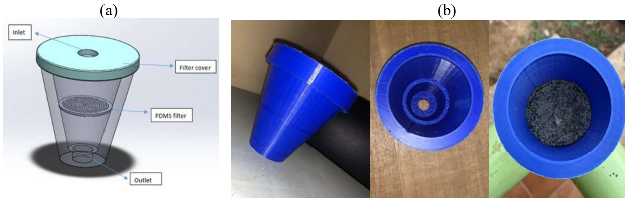
Figure 3.7: a) The Solidworks design of the filter container b) the 3D printed filter container with the PDMS membrane in it.
