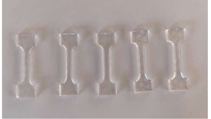
F1: Dogbone mould for the tensile strength testing of PDMS samples.
