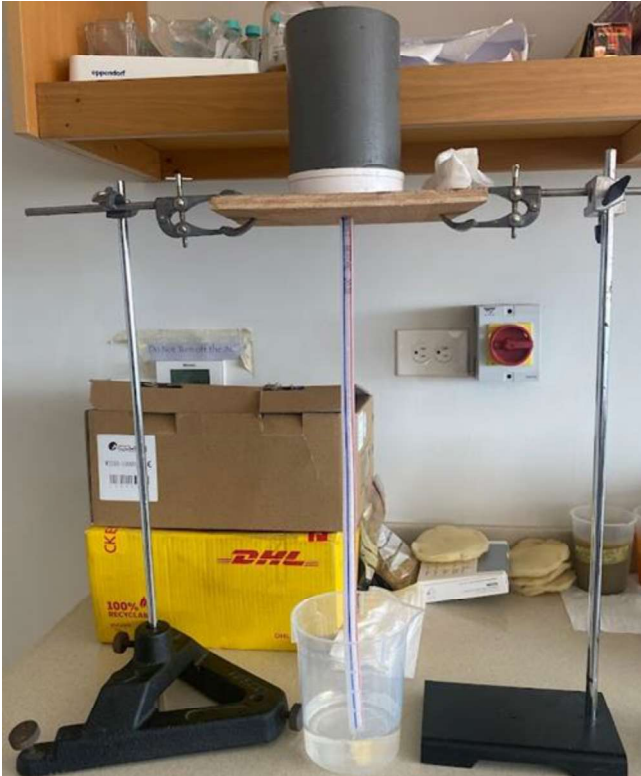
A1: Experimental setup for control test using commercial activated carbon
