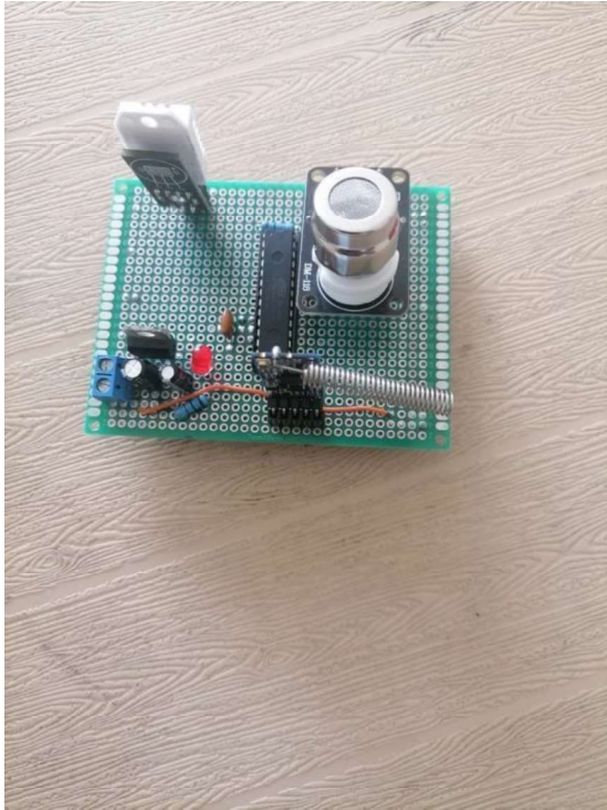
Figure 4.11: Perforated board implementation of sensor node 2
