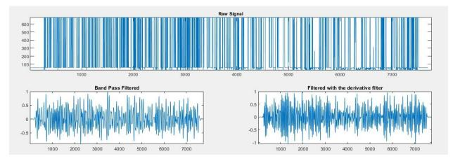
Figure 5-3. Pulse sensor-generated signals before and after each stage of filtration
