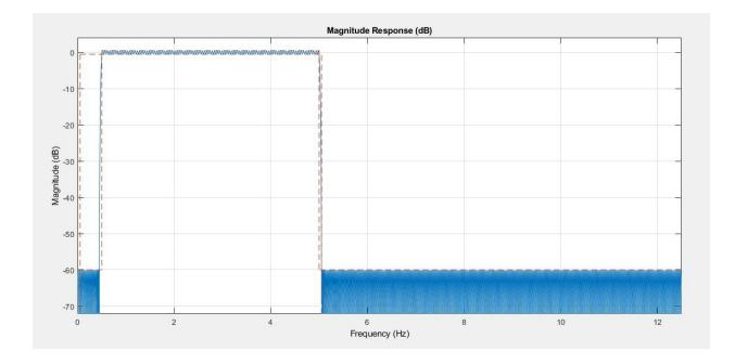
Figure 4-5. Magnitude response of the FIR bandpass filter
