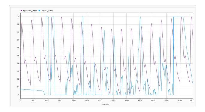
*Figure 5-4. Plot of synthetic PPG signal and PPG signal generated from the pulse sensor*
