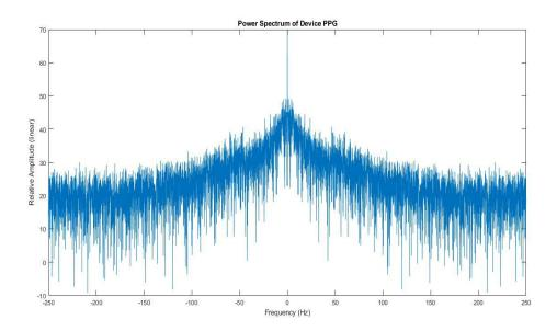
Figure 5-5. Power spectrum of pulse sensor-generated PPG signal
