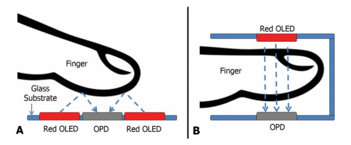
Figure 4-4. Set up to obtain a PPG signal from a pulse sensing device. (A) Reflective mode; (B) Transmissive mode [20].
