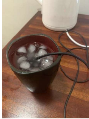
Figure 4.0 7: Temperature sensor immersed in ice bath
