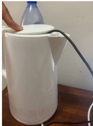
Figure 4.0 6: Temperature sensor immersed in boiling water
