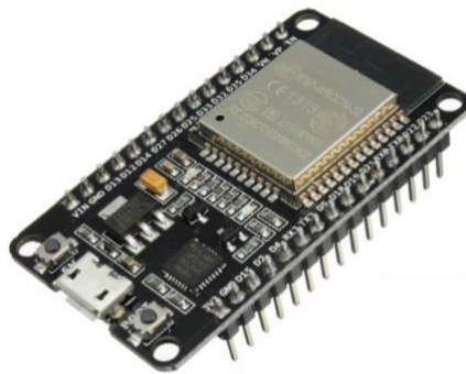
Figure 3.1: NodeMCU ESP32 (ESP-WROOM-32) microcontroller development board
