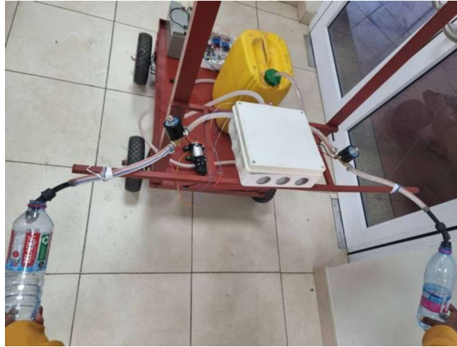
Figure 6.1: Setup for testing flow sensors
