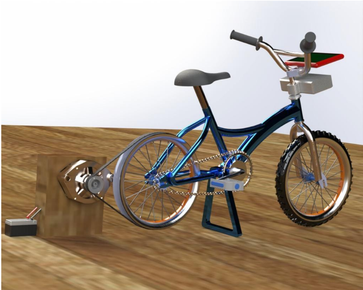
Figure 2: The multipurpose pedaling system design in Solid Works.
