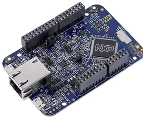
Figure 3.1: FRDM-K64F Development Board with MK64FN1M0VLL12 microcontroller
