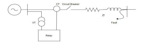
*Figure 2.4 A diagram illustrating line protection using distance relay.*
