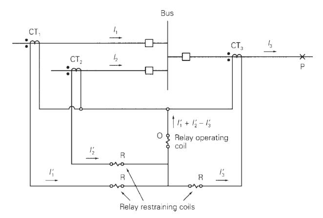
Figure 2.6 A diagram illustrating line protection using differential relay
