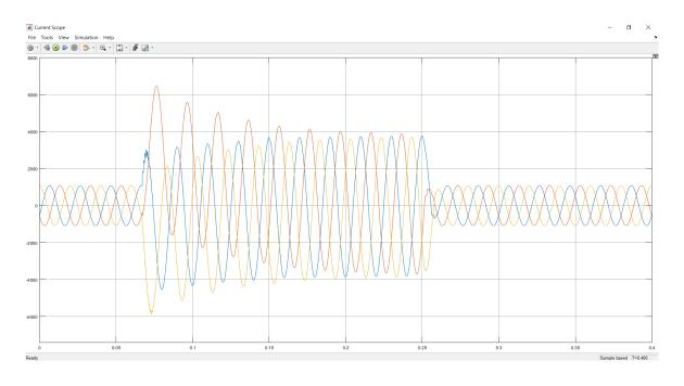
Figure 5.5: Current Output for a Three Phase to Ground Fault
