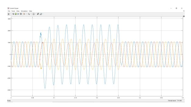
Figure 5.3: Current Output for a SLG fault
