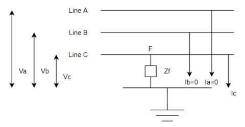
Figure 2.1 A diagram of Line to ground Fault
