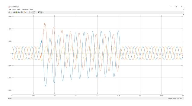
Figure 5.4: Current Output for a DLG fault
