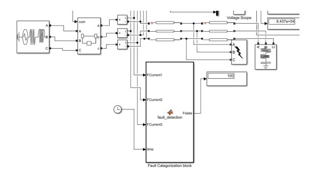
Figure 5.10: Diagram illustrating SLG Fault Categorization
