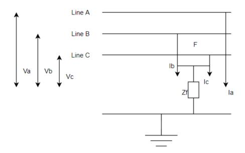
Figure 2.3 A diagram of Double-Line to ground Fault
