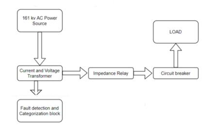
Figure 3.1: Function Block Diagram of Design
