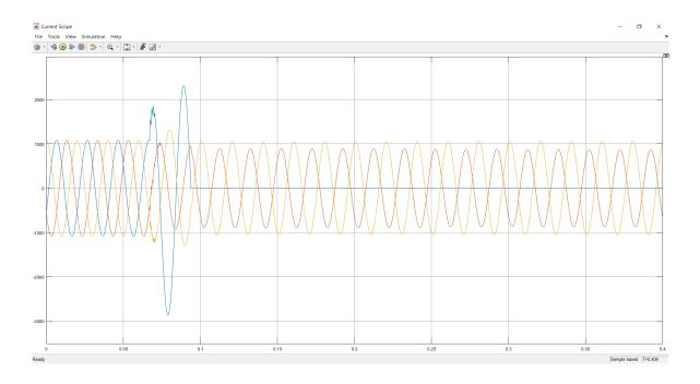
Figure 5.8: Current Output Showing isolation for a SLG Fault
