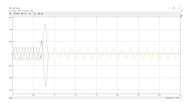
Figure 5.7: Current Output Showing isolation for a DLG Fault
