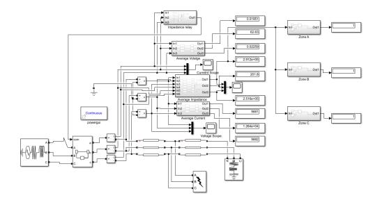
Figure 5.9: Diagram illustrating Fault Detection in Zone C
