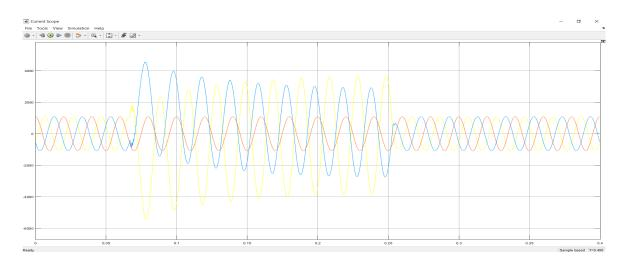
Figure 5.6: Current Output for a Line-Line Fault
