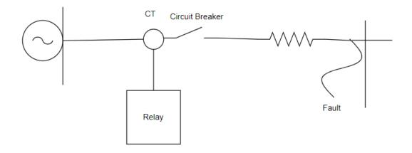
Figure 2.5 A diagram illustrating line protection using over current relay
