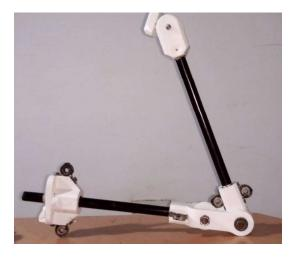
Figure 5.5: Fully jointed arm skeletal unit
