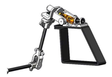
Figure 3.10: CAD model of conceptual design C
