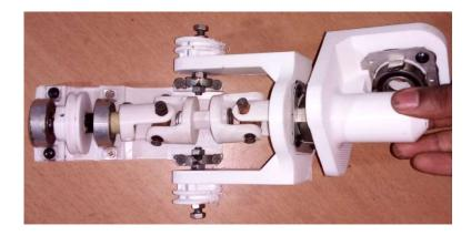
Figure 5.6: Assembled shoulder module top view with shoulder tilted in extension; (From left to right) Shoulder supporting bearings, Shoulder flexion/extension pulley on shoulder, Double cardan joint, Shoulder abduction/adduction socket, Shoulder
