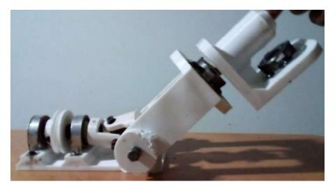
Figure 5.7: Assembled shoulder module side view with shoulder in abduction (elevated); (From left to right) Shoulder supporting bearings, Shoulder flexion/extension pulley on shoulder, Double cardan joint, Shoulder abduction/adduction socket, Shoulder
