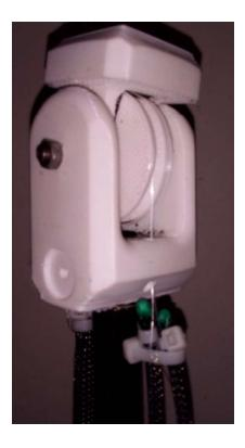
Figure 5.8: A muscle connection to joint pulley system (forearm wrist joint example)
