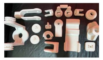
Figure 5.1: 3D-printed lightweight arm joint components
