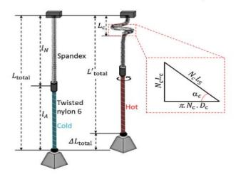
Figure 1: Schematic showing twist coil actator system that is heated to cause rotation.
