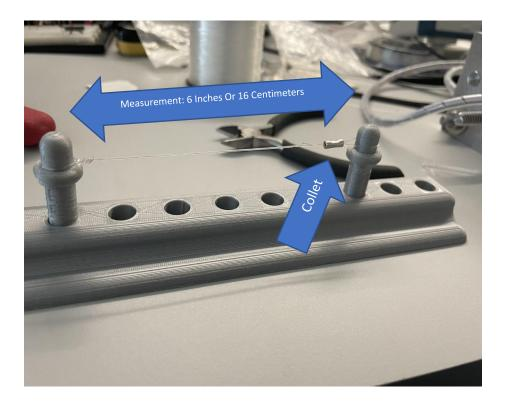
Figure 10: Measurements of the Nylon before twisting
