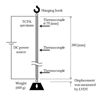
Figure 14: Schematic of TCPA Measurements with LVDT and Core Sensor (Kikuta)
