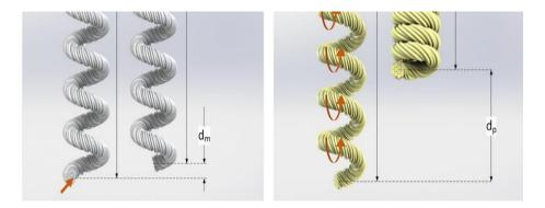
Figure 3: Effect of heat on the length of a metallic helix (left) and TCP (right) [Karami]
