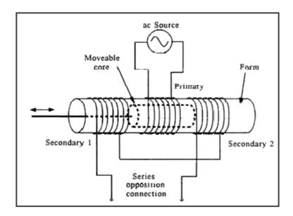
Figure 5: Linear Displacement Measurements [Ni.com]
