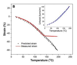
Figure 2: A plot of the tensile actuation measured from the coil vs temperature.
