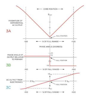
Figure 7: Proportionally linear LVDT Response to Core Displacement
