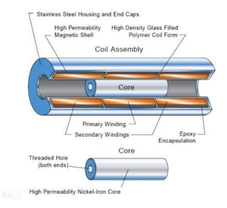
Figure 6: LVDT Sensor With the Core [NI.com]
