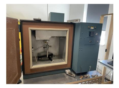
Figure 12: The heating Chamber for the Annealing process
