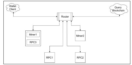
Fig. 17. Network architecture revision, adding a peer called RPC3 to the hardware running the attacker, Miner1.
