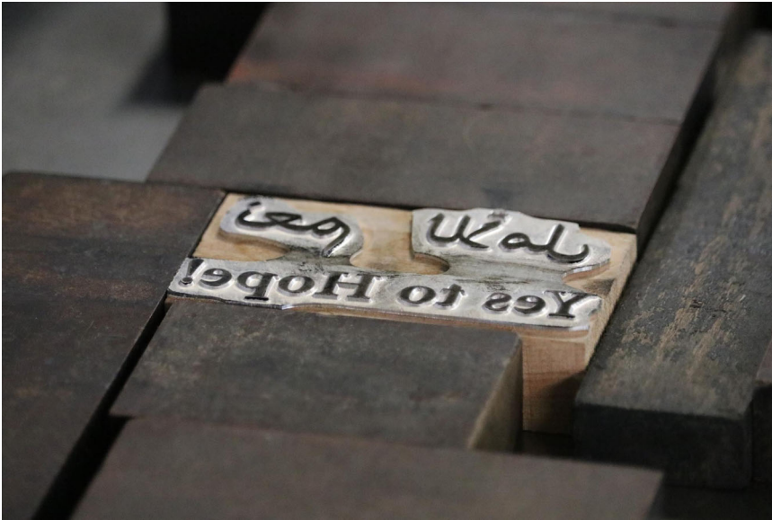
Figure 2. Custom letterpress plate used to print the title on covers of Yes to Hope! (2018). Photo credit: Hussam Al-Obaidi.
