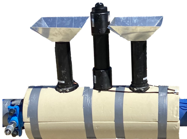
Figure 8. Complete device mounted on a water pipe with attached insulation.
