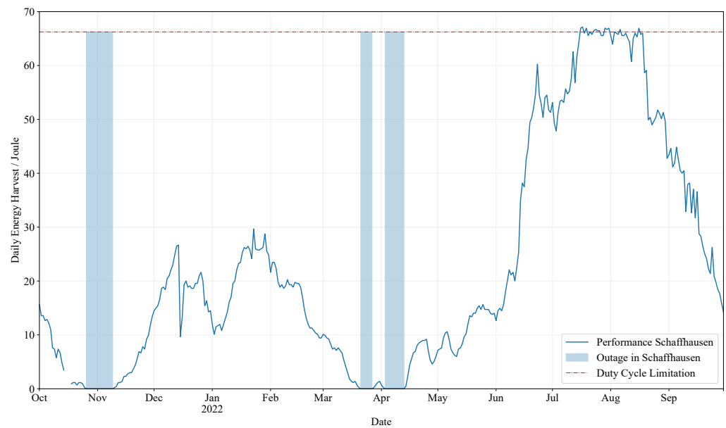
Figure 12. Daily energy harvest of the buried device during the field test in Schaffhausen: The daily energy harvest equals the number of daily uplinks multiplied by the energy required for a single uplink. The red line shows the limitation due to the duty cycle restrictions imposed by LoRaWAN. Coloured areas show outage days, i.e., days without uplinks from the harvesting device. The missing data points are due to technical problems with the LoRaWAN gateways. The data from the harvesting device in Winterthur are available in Appendix A.2 (Figure A1).
