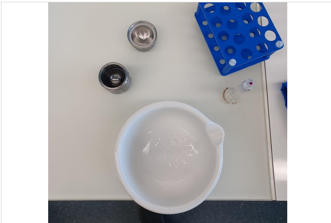
7.1.1 Frozen MeCN to simulate the cryomill step while evaluating potential contamination sources.
