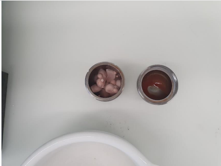
6.1.2 O. mykiss liver sample had to be pre-frozen in a mortar bowl to prevent the grinding ball and the homogenate from sticking together.
