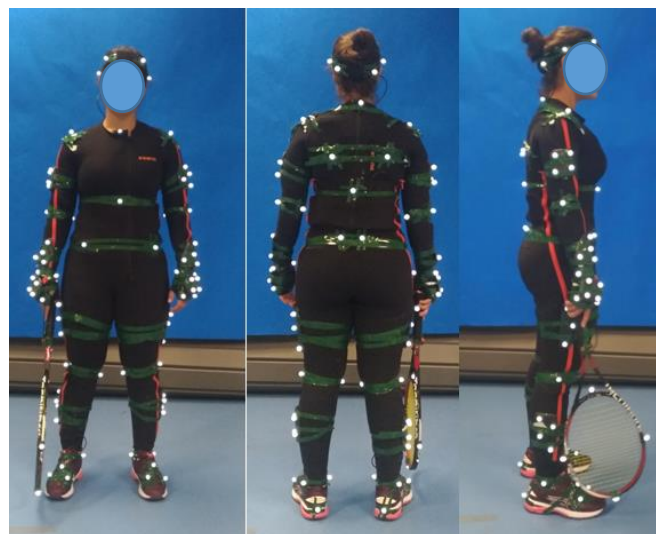
Figure 2.2 - Individual set-up. Marker set up placed on each body segment with 43 reflective markers and 10 lightweights with 4 non-collinear tracking markers.
