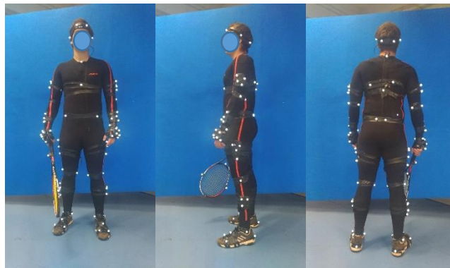
Figure 5.2 – Marker set-up. 43 reflective markers and 10 lightweights with 4 non-collinear tracking markers.
