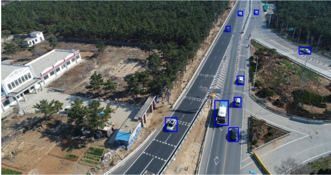
Figure 1.1: RGB UAV image with bounding boxes of vehicles overlay in blue.
