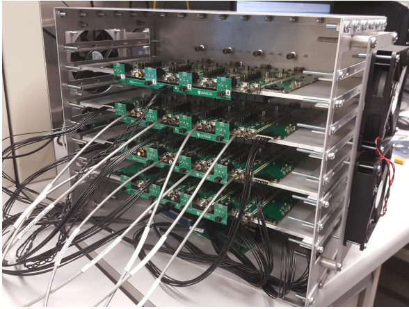
(a) RF front-end showing 4 blades, each housing 4 two-stage PAs.
