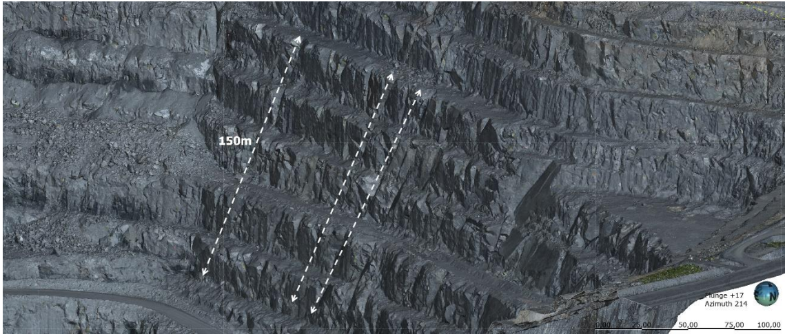
Figure 58. 3D view of the 2022 pit photogrammetry. Persistence of structures from Set E and Set F in the western wall of the pit.
