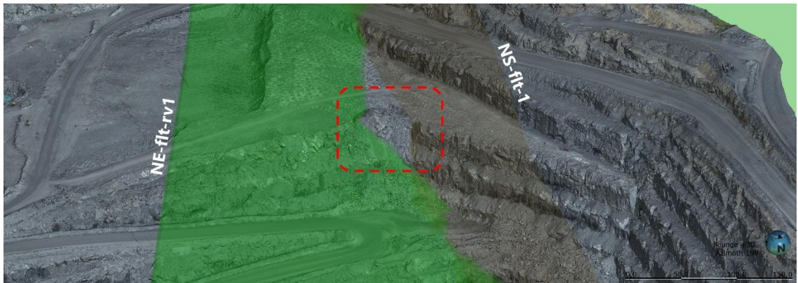
Figure 116. Wedge failure in the southwest section of the pit. From 3D photogrammetry.
