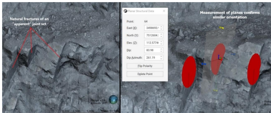
Figure 37. Procedure for measuring structural planes in LeapfrogGeo 2021.2.5
